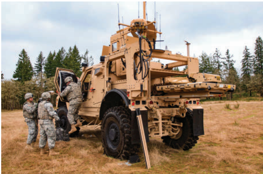
The U.S. Army Prophet Enhanced tactical signals intelligence and electronic warfare system relies on several different RF transmitters and receivers to gather crucial battlefield information.
