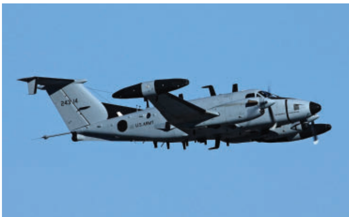
The U.S. Army RC-12 Guardrail special electronic mission aircraft must pack together many different RF antennas on this small twin-engine plane.
