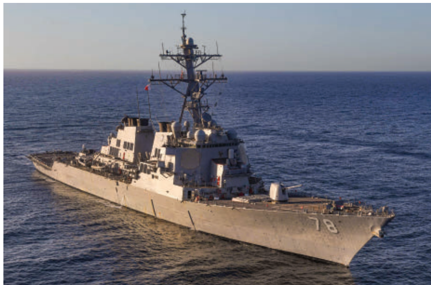
The U.S. Navy's Arleigh Burke-class guided missile destroyer must accommodate a wide variety of RF systems and antennas, all crowded tightly together on the ship's masts and superstructure.
